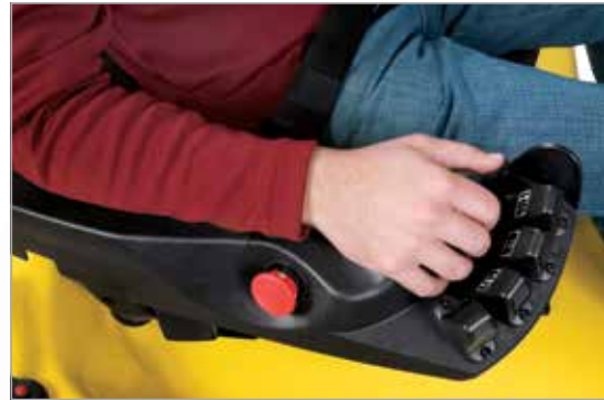
Electro-hydraulic controls with TouchPoint mini-levers
