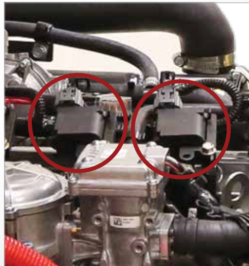
Coil over plug ignition design
