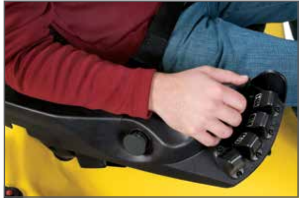
Electro-Hydraulic Controls with TouchPoint Mini-Levers
