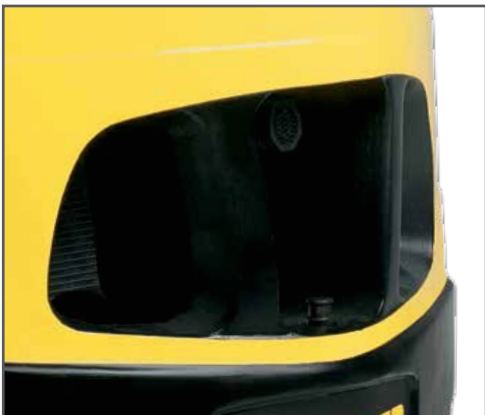
Counterweight tunnel design improves airflow
