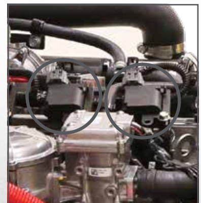
Coil over plug ignition design
