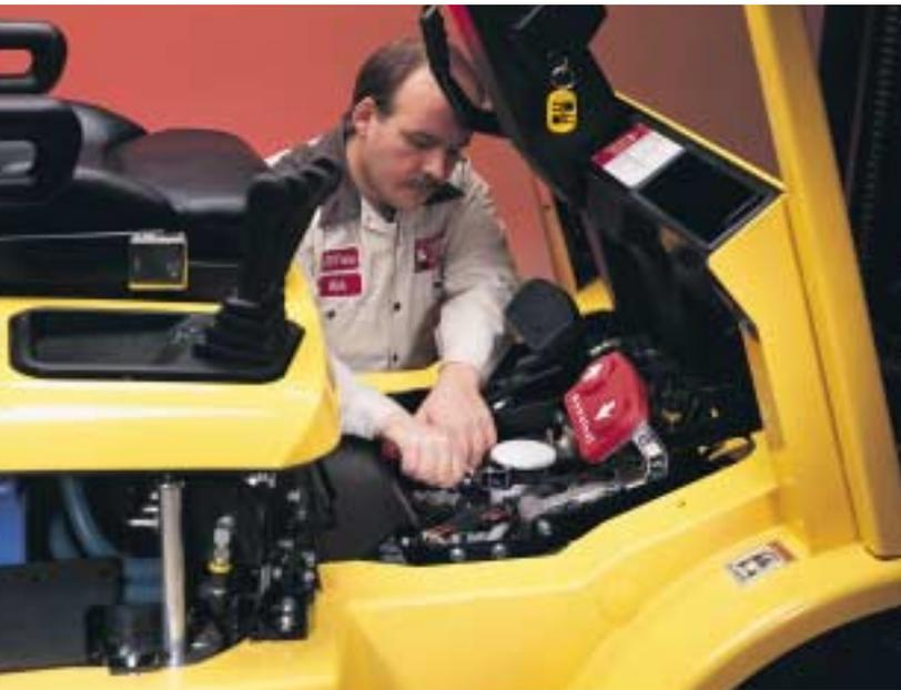
**▶** Plenty of room to work. Remove the two-piece floorplate and you'll have complete access to the transmission filter and main transmission control valve. A spin-on transmission oil filter gives you "quick change" capability.
