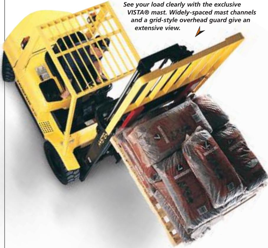
See your load clearly with the exclusive VISTA® mast. Widely-spaced mast channels and a grid-style overhead guard give an extensive view.
