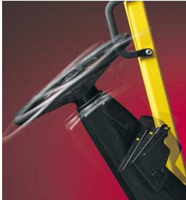
▲ *The new tilt steering column conforms to your driving style. A unique latch specially contoured for quick fingertip access lets you adjust the column to one of four comfortable positions. Power steering response is smooth, sure and takes only 3.7 turns to go lock-to-lock.*
