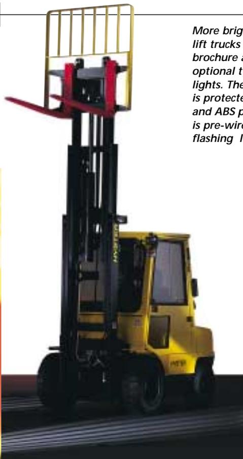
More bright ideas. The H45-65XM lift trucks shown throughout brochure are equipped with the optional two stop and back-up lights. The high-quality light cluster is protected by a plastic housing and ABS plastic cage. The lift truck is pre-wired for added driving or flashing lights. ▼
