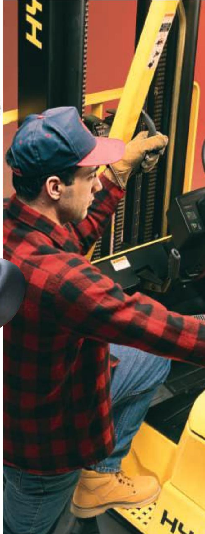
No matter how you grip the 'soft touch' hydraulic levers, they'll mold to your hand for a perfect fit. They're located seat-side where your hand can naturally reach and control the levers, even with your fingertips. Optional fourth function lever shown.
