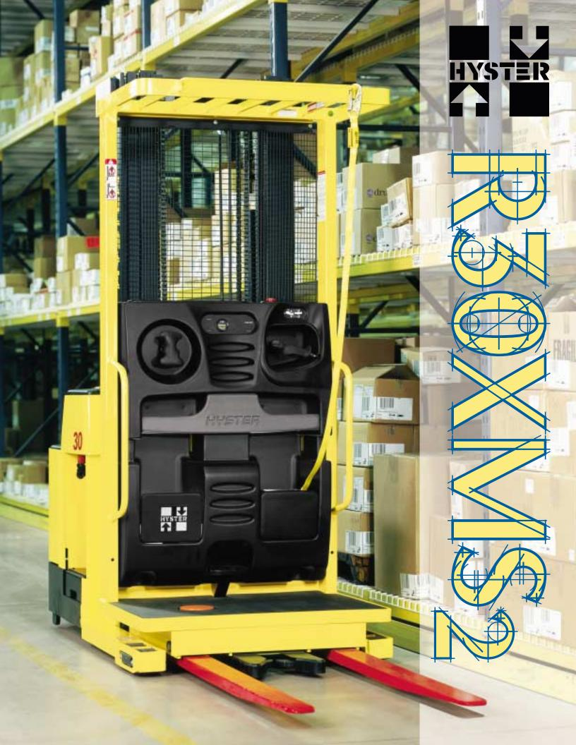
To help your operations reach their full pick potential, the new Hyster R30XMS₂ OrderPicker truck is equipped (standard) with HySense<sup>™</sup>. This control system provides you with a smooth, gradual linear reduction (1 mph every 22.5" in lift height between lift heights of 60.0" and 150.0") that is barely noticeable to your operators for optimized order picking productivity.
