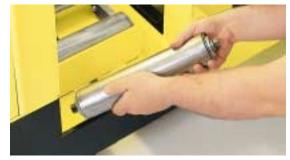
Simple battery access saves you time and money. The R30XMS<sub>2</sub> battery compartment is accessible from both sides through convenient, easily removed side panels. Large, 2.5-inch diameter rollers (optional) allow easy battery access for maintenance checks. Teflon-sealed rollers can be replaced individually.
