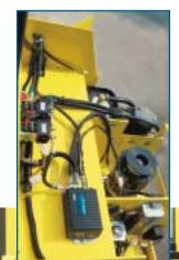
The R30XMS<sub>2</sub> Control Area Network (CANbus) communication reduces the mast conductor wiring to only 8 strands for any combination of options providing you increased reliability.
