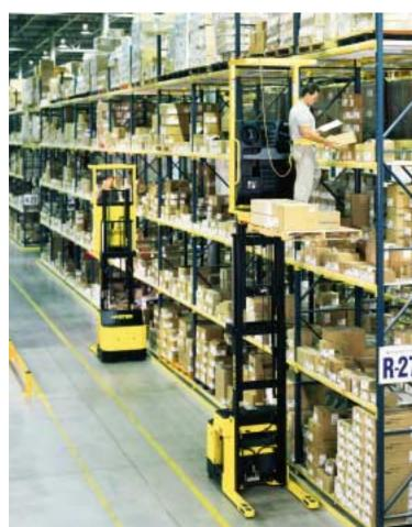
Supporting a variety of pallet sizes is easy. The Hyster R30XMS<sub>2</sub> OrderPicker's pin-mounted adjustable forks and rigid pallet clamp provides centered, secure load handling. A foot-operated lever releases the pallet with ease.
