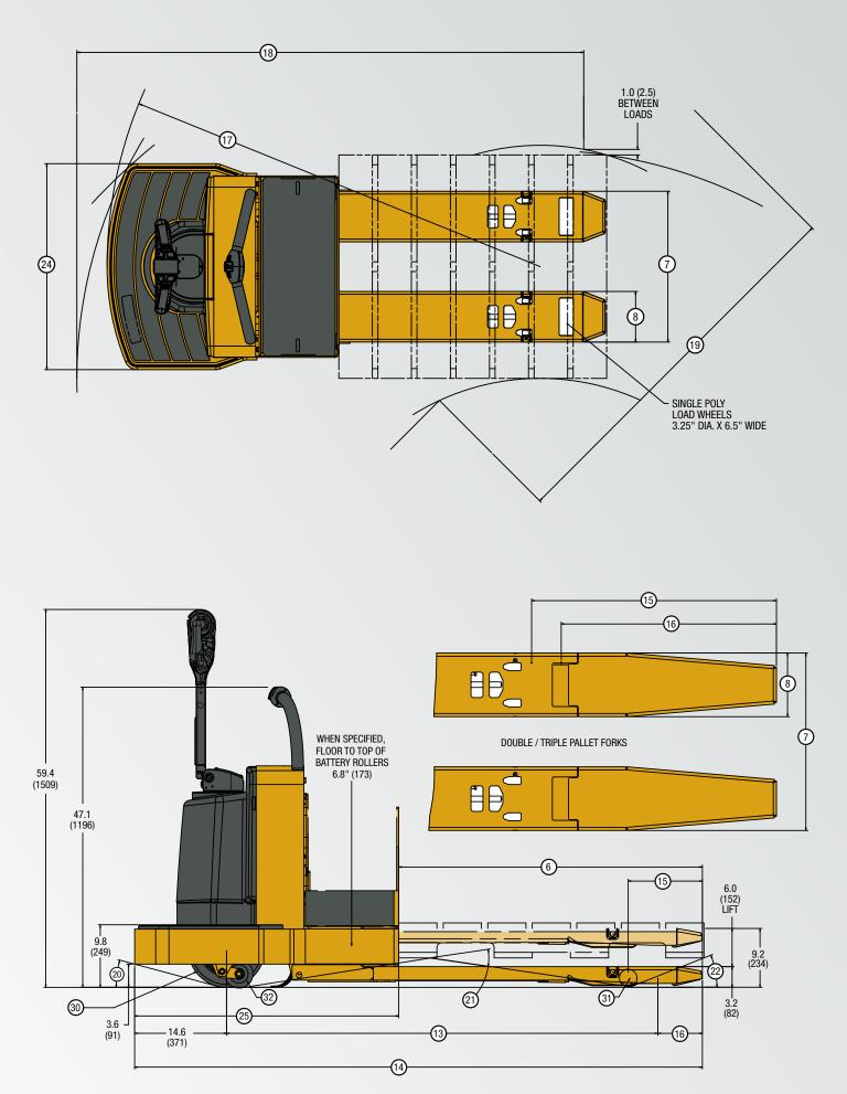
Circled dimensions correspond to the line numbers on the tabulated chart inside the spec sheet. Dimensions are in inches (millimeters).
