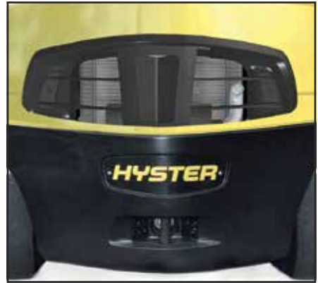
Counterweight venting improves airflow
