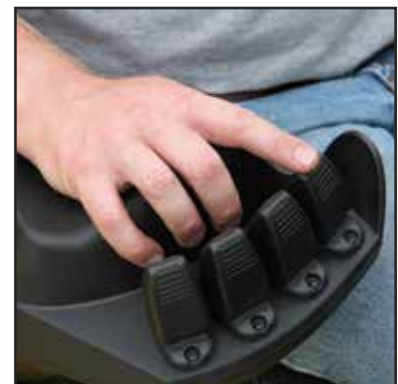
TouchPoint mini-lever electro-hydraulic controls
