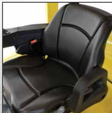
Full suspension swivel seat
