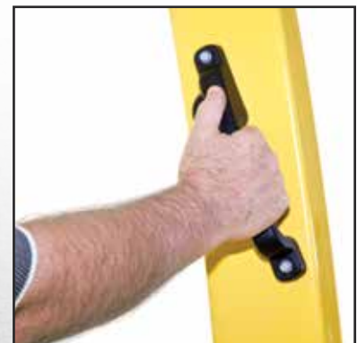
Rear drive handle with horn button
