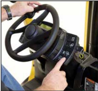
Infinitely adjustable steer column
