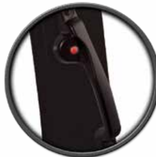
Optional rear drive handle with horn button
