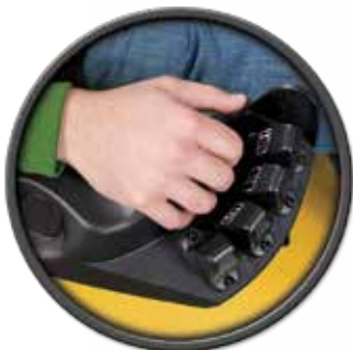
Optional Accutouch mini-lever electro-hydraulic controls with on-demand hydraulics
