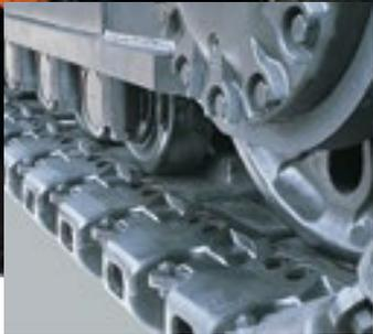
■ Rugged track links include roller guides to help extend service life.
