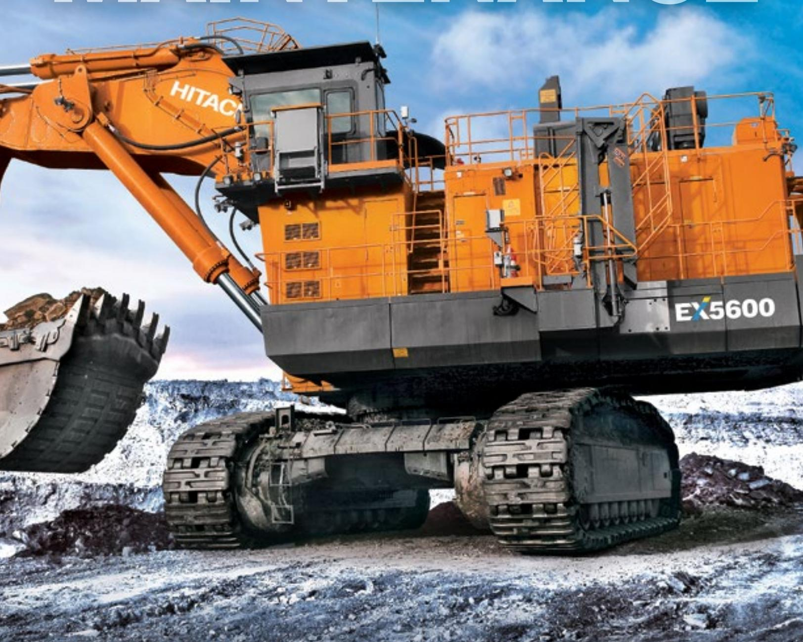
■ A walkway around the entire counterweight provides easy access to rear areas for faster, safer inspections and maintenance.
