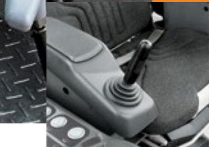
■ Electric joystick control levers provide precise and almost effortless operation.
