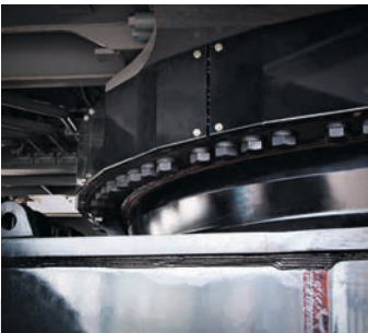
LUBRICATION PIPING COVER A swing circle cover has been added to the outside of the swing bearing, protecting the lubrication piping from debris damage.
