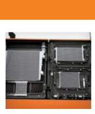
■ Parallel Arrangement of Radiator and Oil Cooler. The radiator and oil cooler are arranged side by side to increase cooling efficiency. This also reduces cleaning time and effort remarkably.
