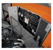
■ Wide-Open Inspection Doors. Inspection doors open wide for easy maintenance.
