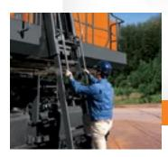
An optional slide ladder gives the operator even easier access to the cab and working platform.
