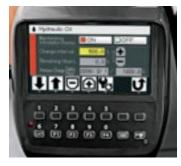
■ The multifunction, multilanguage LCD monitor is easy to read and provides key data about the excavator. The MIC mining system uses a data logging unit to record daily operating conditions and warnings. The monitor can be preset to indicate replacement intervals for engine oil, hydraulic oil and filters.
