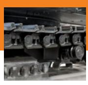
■ Track links are enlarged to increase strength for higher durability and reliability especially on rugged ground.
