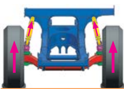
BOTH STRUTS IN COMPRESSION WITH NO HORIZONTAL DEFLECTION
