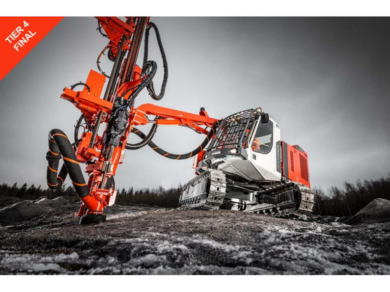
Ranger DX800 is a hydraulic, self-propelled, self-contained, crawler based surface drilling rig equipped with a cabin (F.O.P.S. and R.O.P.S.) and rod handling system.
