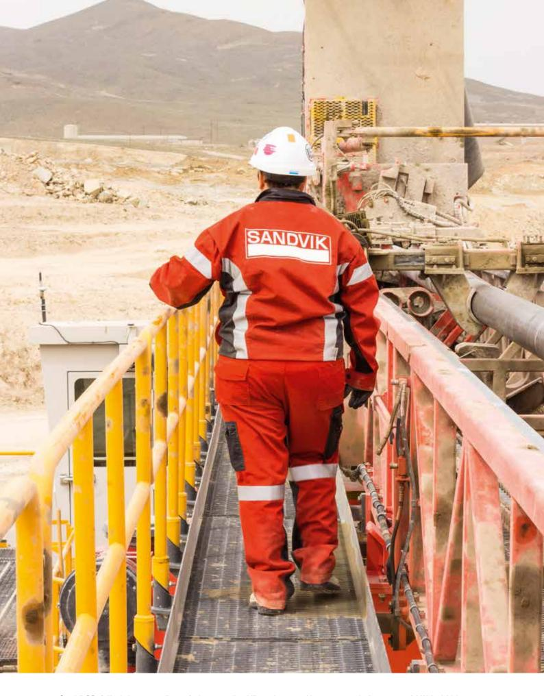
$Sandvik\,DR461i\,includes\,more\,walk ways\,for\,better\,service ability\,and\,access\,with\,open\,serrated\,grip\,strut\,material.\,We've\,laid\,the\,grating\,in\,the\,direction\,of\,foot\,traffic\,to\,enable\,mud\,to\,fall\,through.$
